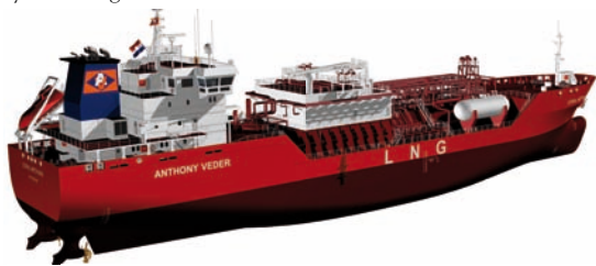
The model shows Coral Methane's pair of Azipull 120 thrusters with pulling propellers
